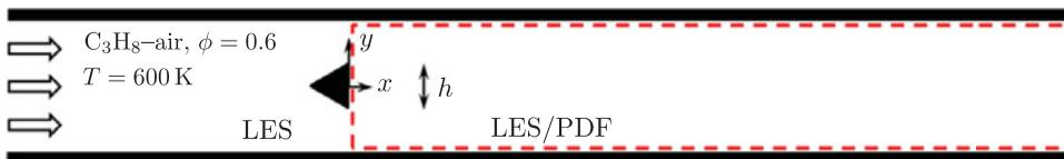
Figure 1. A schematic diagram for the computational domain on the  $x$ - $y$  plane. (Colour online.)
