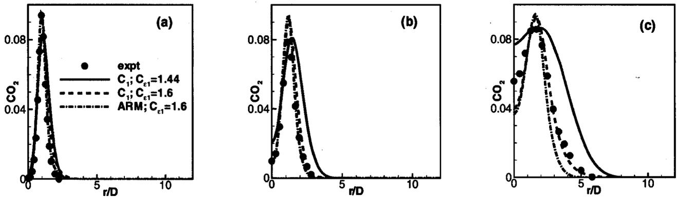
Fig. 4 Radial profiles of mean  $\text{CO}_2$  mass fraction; (a)  $X/D=7.5$ , (b)  $X/D=15$ , and (c)  $X/D=30$
