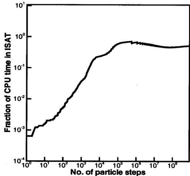
Fig. 15 Fraction of the CPU time spent in ISAT for the jet diffusion flame
