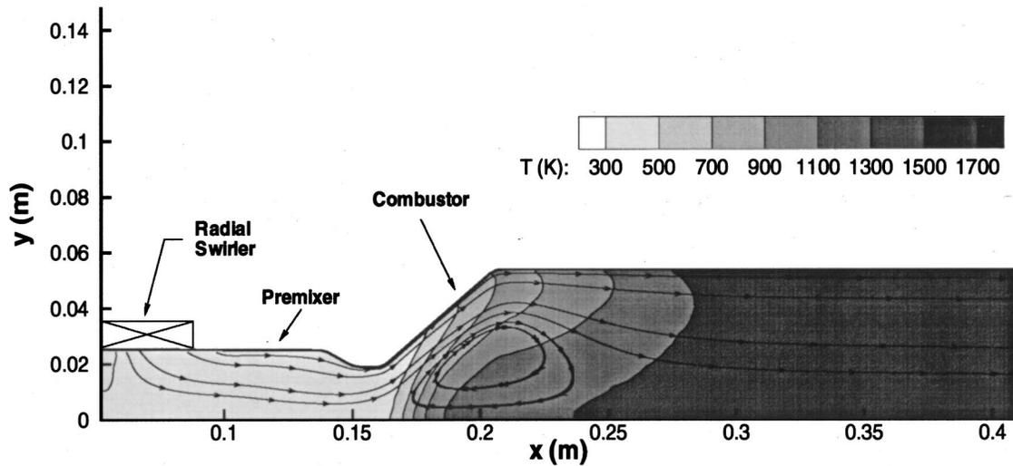
Fig. 12 Contours of the Favre mean temperature and sample steamtraces in the premix combustor
