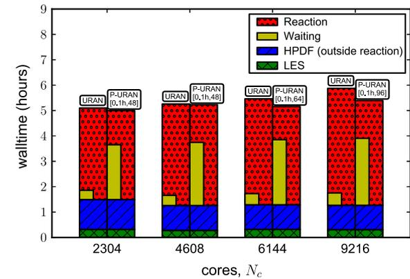
**Fig. 10.** Weak scaling tests using the URAN and P-URAN strategies with the 38-species mechanism (test details provided in Table 2) for  $N_t = 1000$  time steps. Top: weak scaling – wall clock time per time step spent in LES, HPDF (outside reaction), Reaction and Overall. Bottom: breakdown of wall clock time spent in LES, HPDF (outside reaction), Reaction (including  $x2f\_mpi$  communication) and Waiting (average idle time).
