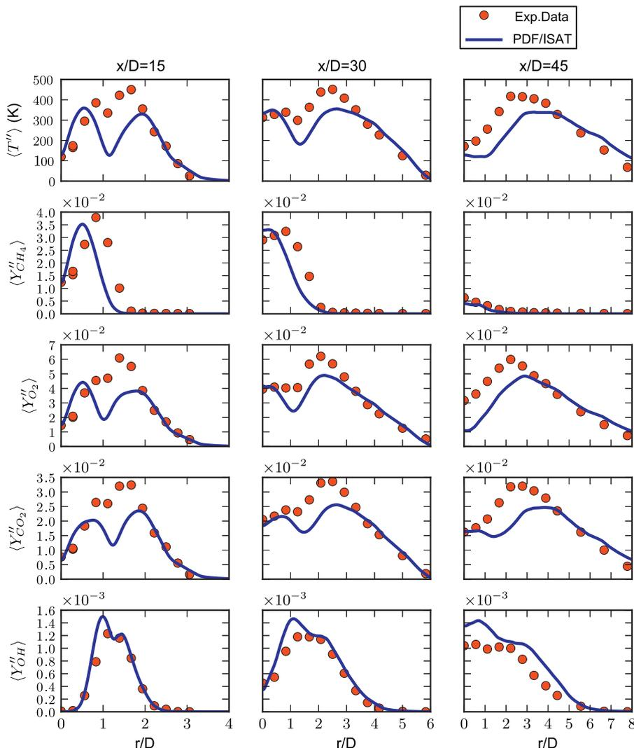
**Fig. 4.** Radial profiles of time-averaged density-weighted standard deviation of temperature  $T$ , and mass fraction of species  $CH_4$ ,  $O_2$ ,  $CO_2$ ,  $OH$  at axial locations  $x/D = 15, 30, 45$  obtained from experimental data and an LES/PDF simulation using the 38-species mechanism.
