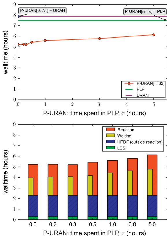
**Fig. 7.** P-URAN sensitivity tests with the 16-species mechanism. Top: wall clock time for 2000 time steps with (i) PLP; (ii) URAN; and (iii) P-URAN[ $\tau$ , 32] with time  $\tau$  spent in PLP varied from 0 to 5 hours. Bottom: breakdown of wall clock time spent in LES, HPDF (outside reaction), Reaction (including  $x2f\_mpi$  communication) and Waiting (average idle time) in the P-URAN tests.
