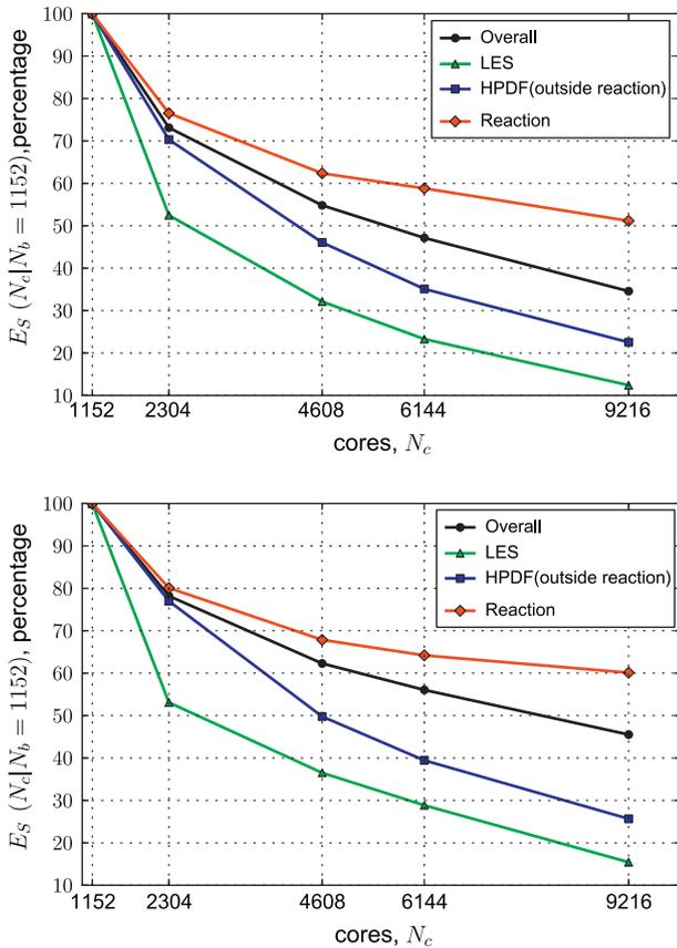
**Fig. 14.** Relative strong scaling efficiency of LES, HPDF (outside reaction), Reaction and Overall using the P-URAN strategy. Top: with the 16-species mechanism for a simulation of  $N_t = 2000$  time steps. Bottom: with the 38-species mechanism for a simulation of  $N_t = 1000$  time steps.
