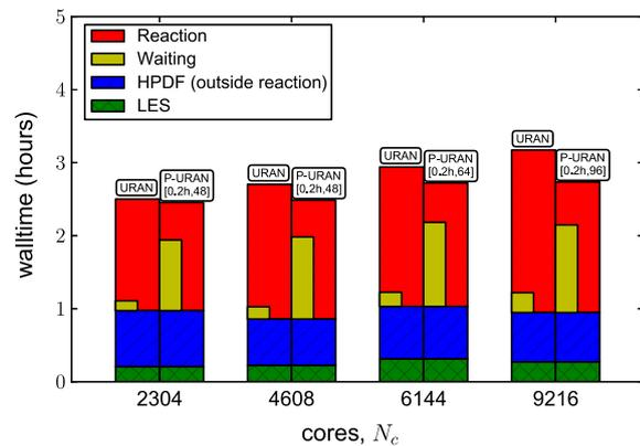
**Fig. 9.** Weak scaling tests using the URAN and P-URAN strategies with the 16-species mechanism (test details provided in Table 2) for  $N_t = 1000$  time steps. Top: weak scaling – wall clock time per time step spent in LES, HPDF (outside reaction), Reaction and Overall. Bottom: breakdown of wall clock time spent in LES, HPDF (outside reaction), Reaction (including  $x2f\_mpi$  communication) and Waiting (average idle time).
