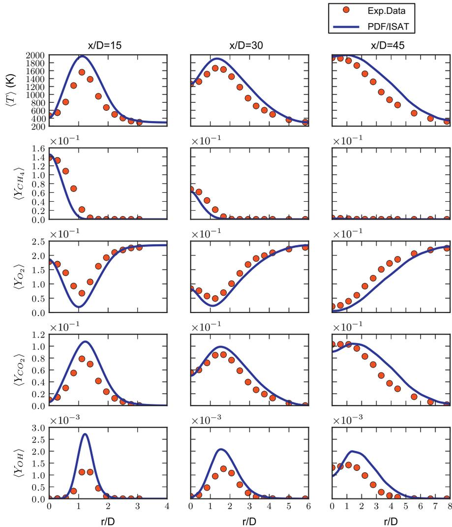
**Fig. 3.** Radial profiles of time-averaged density-weighted mean temperature  $T$ , and mass fraction of species  $CH_4$ ,  $O_2$ ,  $CO_2$ ,  $OH$  at axial locations  $x/D = 15, 30, 45$  obtained from experimental data and an LES/HPDF simulation using the 38-species mechanism.
