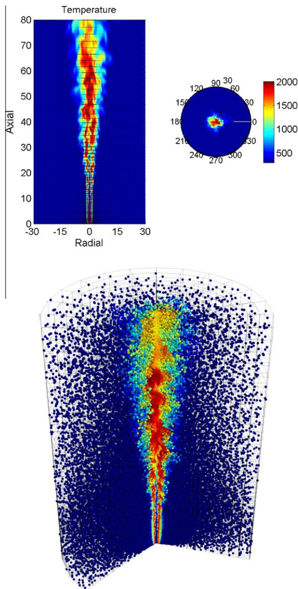
**Fig. 1.** LES/PDF simulation of the Sandia Flame D. Top: Instantaneous temperature distribution on a 2D cut-plane through the axis of the computational domain. Dots in the plot indicate every third grid node in the axial and radial directions. Bottom: A 3D slice-view of the PDF particle temperature distribution in the computational domain. Every fourth LES grid line is shown.
