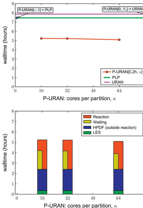
**Fig. 8.** P-URAN sensitivity tests with the 16-species mechanism. Top: wall clock time for 2000 time steps with (i) PLP; (ii) URAN; and (iii) P-URAN[0.2 h,  $\kappa$ ] with the partition size,  $\kappa = 16, 32, 64$ . Bottom: breakdown of wall clock time spent in LES, HPDF (outside reaction), Reaction (including  $x2f\_mpi$  communication) and Waiting (average idle time) in the P-URAN tests.
