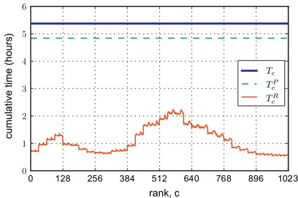
**Fig. 15.** LES/PDF simulation of the Sandia Flame D for  $N_t = 2000$  time steps on  $N_c = 1024$  cores with chemistry represented using the 16-species mechanism with the P-URAN[0.2 h, 32] parallel strategy. On each core ranked,  $c = 0-1023$ , plotted are the cumulative wall clock time spent on the computations,  $T_c$ ; the part of the time spent within HPDF,  $T_c^P$ ; and within HPDF the part of the time spent on Reaction (including  $x2f\_mpi$  communication),  $T_c^R$ .
