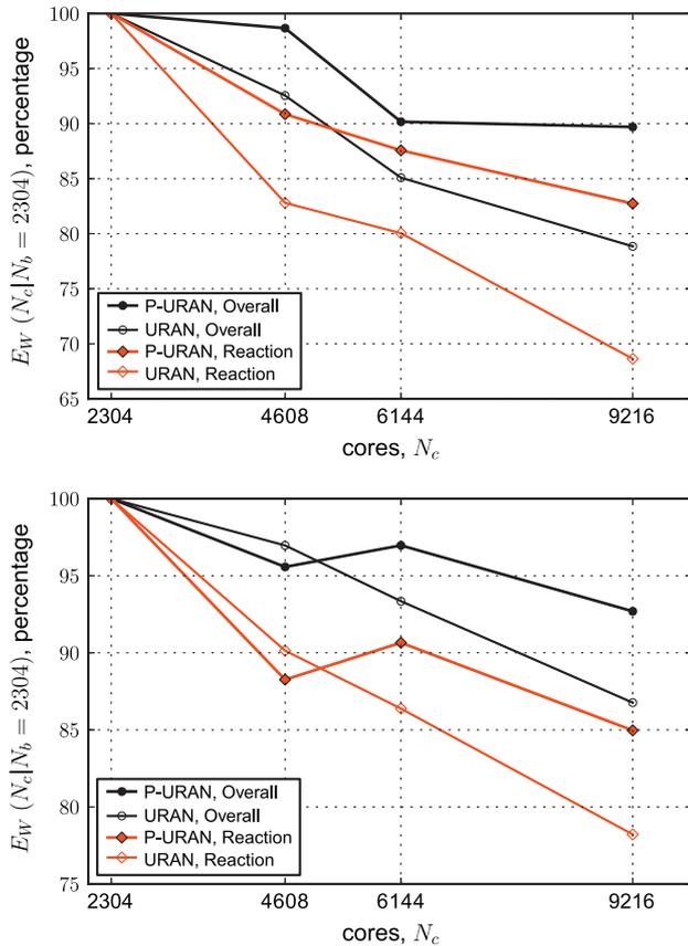
**Fig. 11.** Relative weak scaling efficiency of Reaction and Overall using the URAN and P-URAN strategies. Top: with the 16-species mechanism for a simulation of  $N_t = 1000$  time steps. Bottom: with the 38-species mechanism for a simulation of  $N_t = 1000$  time steps.
