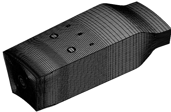
Figure 6. The computational grid of Combustor-B. Air is fed through swirlers and primary, dilution and effusion holes. The grid has 400,752 nodes.
